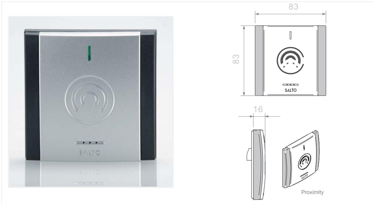
SALTO modular wall readers WRM9000 and WRM9001 read & write information on contact less smart cards (RFID) compatible with ISO 14.443A, ISO 14.443B and ISO 15.693 (VICINITY) standards, and as MIFARE, DESfire or VICINITY technologies. They also allow for updating of the carriers via the SALTO Virtual Net (SVN) technology.
