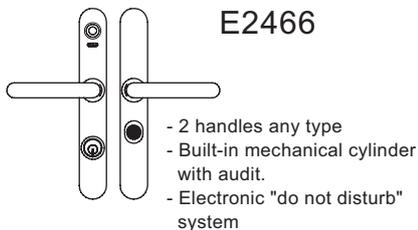
**Outside handle:** Free floating system, which connects the handle when access is granted.
