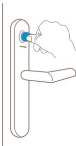
Just by touching the i-Button on the reader, the electronic handle turn will grant or deny the access to the door giving an acoustic and visual signal and in addition:
